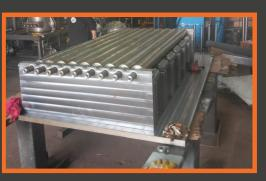
Reversible flattening rollers extend the service life of the roller and minimize wear. The rollers can be easily taken out and cleaned with the help of a motorized stand.
