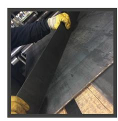
The roller flattening machine reduces the internal tension of sheet metal parts coming from laser cutting, allowing them to straighten. Processes such as precision welding, bending and twisting after straightening are improved. Compared to other flattening processes, cylindrical sheet flattening is fast, economical, short-lived, simple and can be performed with a short training in terms of technical personnel.
